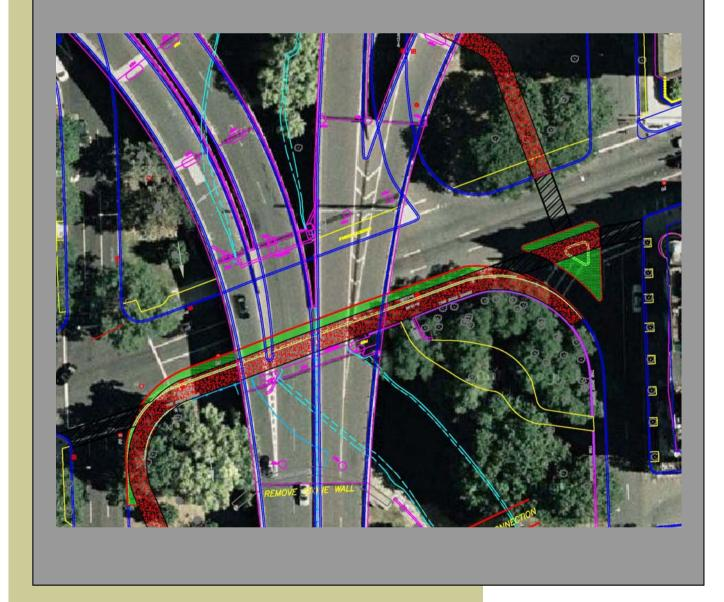
2) Design of an embankment along the onramp to Bowker Overpass near Commonwealth Ave East
